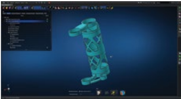
Figure 4: MSC Apex topology optimization of the folding bike fork geometry
