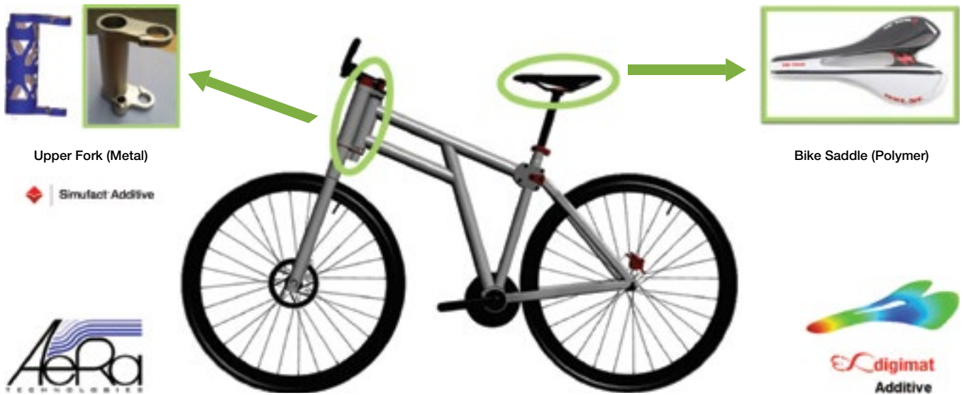
Figure 2: Concept of a folding bicycle with 3d printed Metal and Polymer parts
