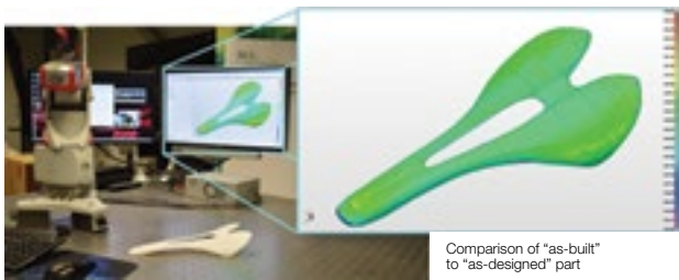
Figure 7: Comparison of the final 'as-built' 3D printed polymer seat part to the 'as-designed' part in Digimat Additive
